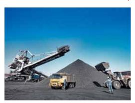
Shipped to the coke plant furnaces via conveyor belts, coal is converted into coke under high temperature and in an oxygen-free environment. This is the procedure of manufacturing coke, deemed necessary by blast furnaces.
