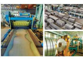
The sized flat steel products ordered by customers are shipped subsequent to being subjected to the slitting and cutting processes at the Steel Service Centers (i.e. ERSEM) located in Gebze, iskenderun and Ereğli.
