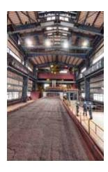
Sinter is produced after fine ore, iron flue dust/fine and oxide are dimensioned to a correct size at the sinter plants so that they can be utilized by the high blast furnaces. Subsequently, they are transferred to the blast furnaces via the conveyor belt system.
