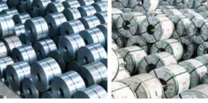
Coils produced at hot rolling mill are rolled in cold rolling mill at room temperature. In this fashion, they are made thinner and a cold product is obtained. Furthermore, depending on demand, the cold rolled products are made into galvanized or tin-chrome coated steel utilized for packaging.
